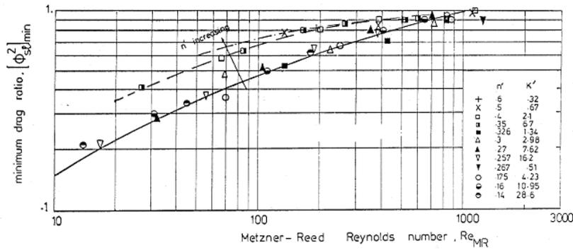
Figure 2. Maximum reductions in frictional pressure loss attainable for a power law slurry (Farooqi and Richardson, 1982)
